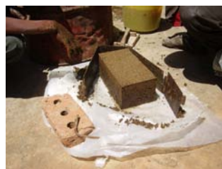
Step 4. Removing block from the mold
