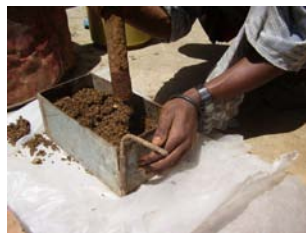
Step 1. Filling the mold
