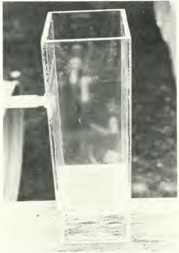
FIG. 4. Mussel holder designed for water ascending up through screen on which mussels rest.
